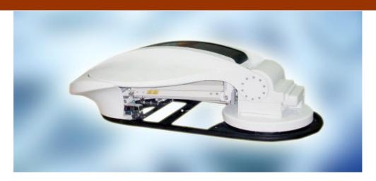
The Drivesat™ AP 770Ka is a fully motorized off set Antenna with a 77 cm reflector and prime focus feed-horn system housed in a POD (Shell) for protection against weather influences and to improve vehicle performance.
