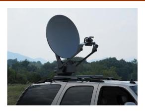
The **DriveSat<sup>TM</sup> AP850** is a transportable system especially designed for multimedia applications via satellite. In particular, this station is compatible with **KA SAT** services..
